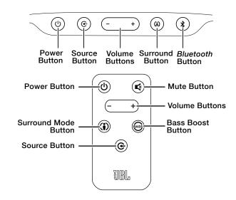
**Power button:** To turn the soundbar on when it is in the Standby mode, press the Power button on either the soundbar or the remote. (The Power indicator will turn white.) To put the soundbar in the Standby mode, press either Power button while the system is on. (The Power indicator will turn amber.) If you do not press the Power button, the soundbar will automatically go into the Standby mode approximately 10 minutes after the audio signal ceases.
