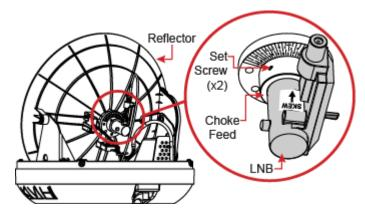
7. Rotate the LNB clockwise or counter-clockwise until the arrow on the LNB points to the correct skew angle printed on the choke feed.
