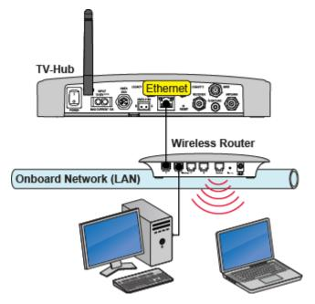
Figure 3-1 TV-Hub Wired Network Connection (TV-Hub A shown)
