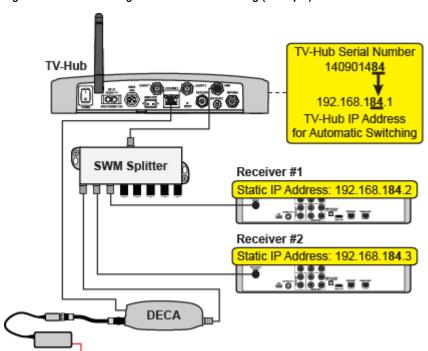
Figure 5-2 IP Addressing for Automatic Switching (Example)
