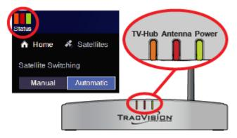
During normal operation, all three lights should be lit green. The following tables explain what the different light conditions indicate. If an error condition exists, view the error message on the Home page of the web interface (see "Error Messages" on page 85).
