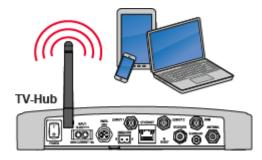
NOTE: If the TV-Hub is connected to an onboard network, you may also access the web interface over the network by entering the TV-Hub's IP address in your browser. (You can find the IP address on the Settings page of the web interface. See "TV-Hub Ethernet Settings" on page 19).
