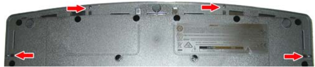
Figure 6. Metal Grille Screw Removal
