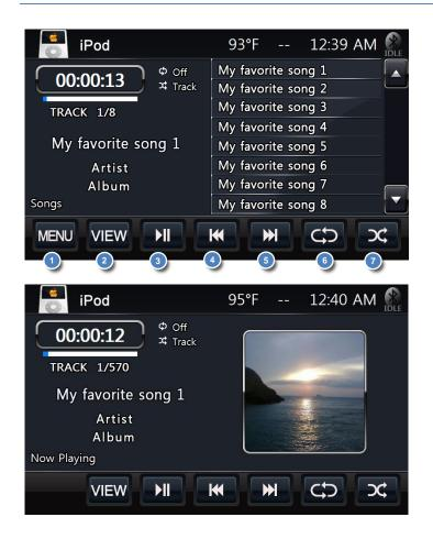
The Infotainment Center can also be connected to your Apple iPod or iPhone. When the iPod is connected, press the **iPod** icon in the Main Menu. The iPod mode can be left any time by pressing the iPod icon at the top left of the screen. To access and use the iPod feature please connect your iPod/iPhone device first to the iPod cable provided.
