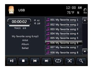
USB mode can be selected from the Main Menu by tapping the **USB** icon on the LCD display. The USB mode can be left at any time by tapping the USB icon at the top left of the USB screen. To access and use the USB feature please connect your USB compatible device (USB stick, HD, etc.) first to the USB cable provided.
