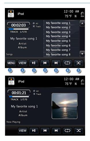
The Infotainment Center can also be connected to your Apple iPod or iPhone. When the iPod is connected, press the **iPod** icon in the Main Menu. The iPod mode can be left any time by pressing the iPod icon at the top left of the screen. To access and use the iPod feature please connect your iPod/iPhone device first to the iPod cable provided.
