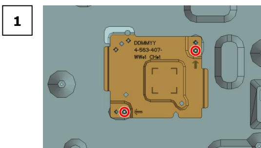
2 screws (SCREW (+PSW) (M3X6)) P/N: 2-990-421-41
