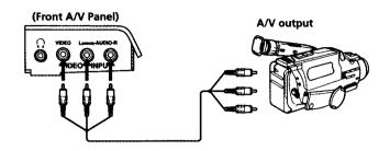
For model KV-13M42, this connection can be made to the AV input located on the rear of the TV.
