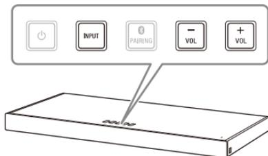
Press **VOL -**, **VOL +**, and **VOL -** in order while pressing and holding **INPUT** on the unit.
