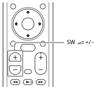
Press **SW (subwoofer volume)**  $\triangle$  +/- to adjust the volume of the subwoofer.
