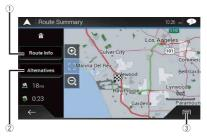
The condition of the displayed route is shown in the upper left by an icon. The total length of the route and approximate required time for the route are in the lower left.
